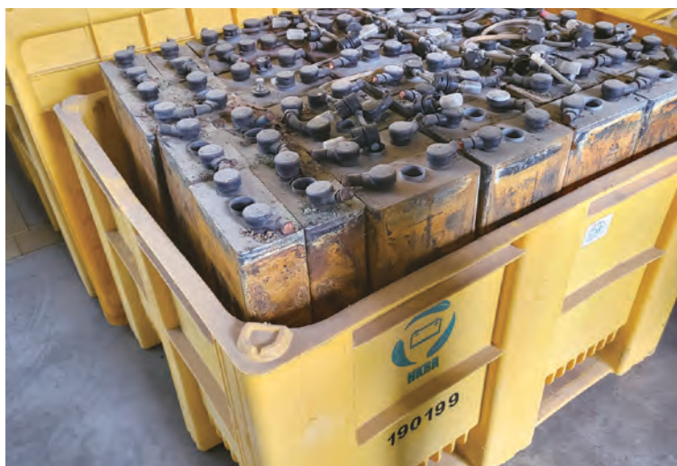
Disused Lead Acid Batteries for Recycling
