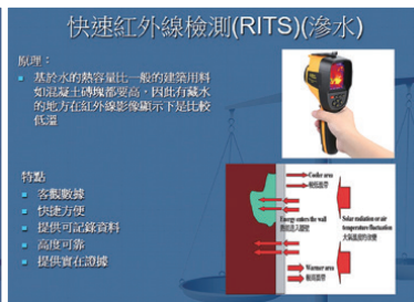
Figure 2: Rapid Infrared Thermographic Survey
